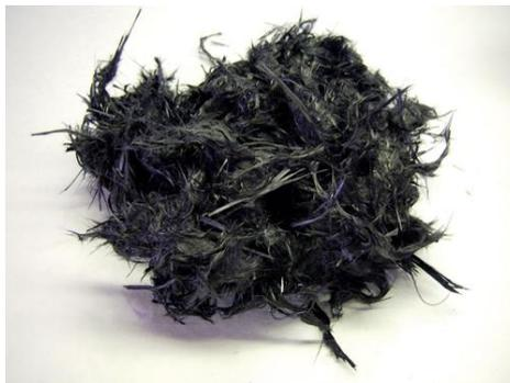
Fig. 1: Recycled carbon fibres in a typical random and fluffy form.
